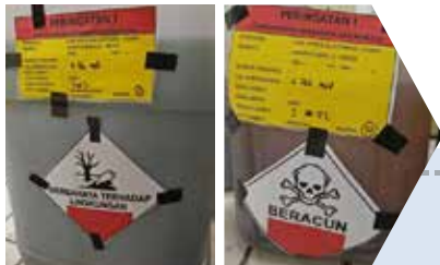
Pengelompokan Limbah B3 di masing-masing Laboratorium B3 waste grouping in each laboratory
